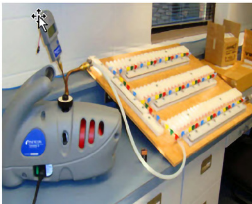
Figure 8. Vials are evacuated of all atmosphere so there is no contamination of sample from ambient air.
