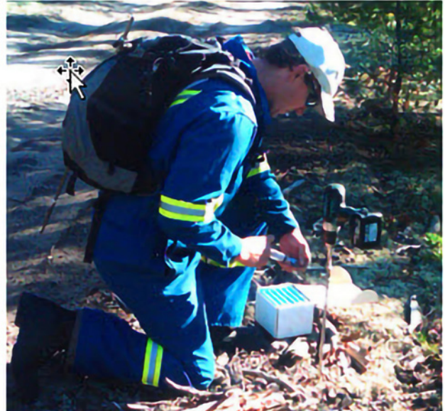
Figure 10. A probe being drilled into the ground in order to collect soil gas sample.
